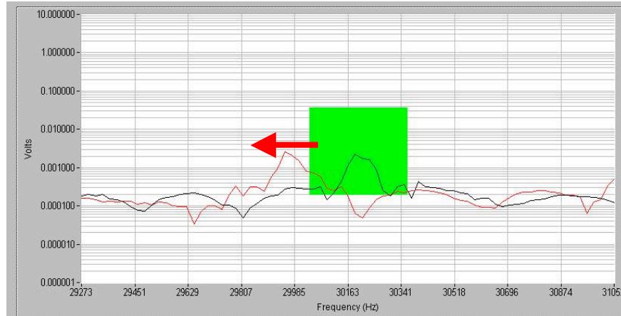
Figure 3. Data showing a typical frequency shift detected by NDT-RAM.
