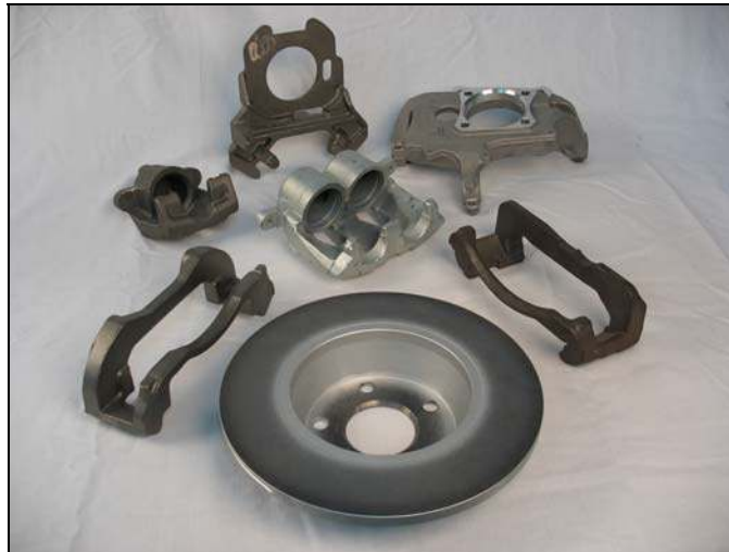
Figure 5 - Sample brake parts commonly inspected for first several natural resonant frequencies via RAM NDT.
