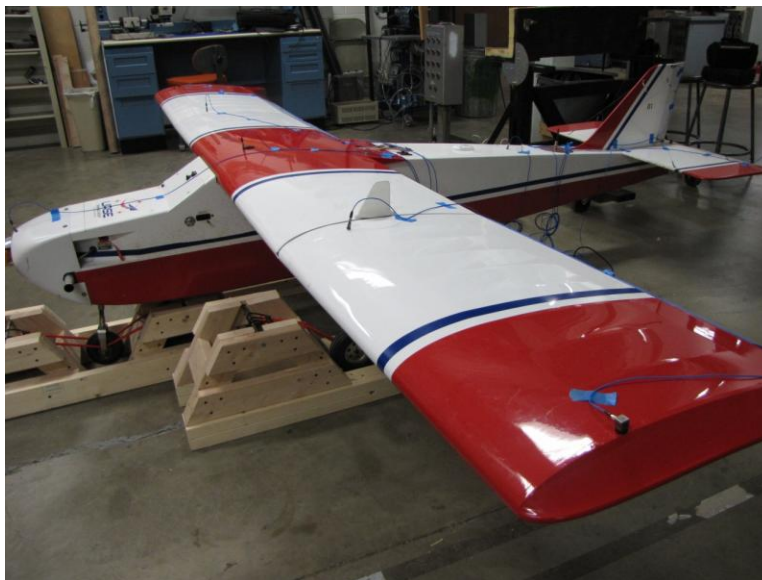
Figure 3. The Super Hauler in the test rig while instrumented with accelerometers.
