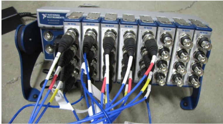
Figure 5. National Instruments cDAQ-9178 data acquisition board used for the testing
