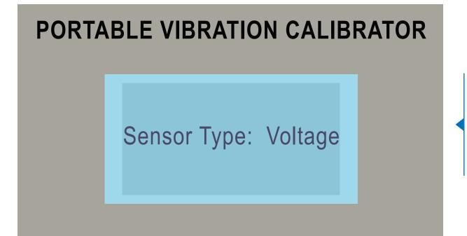
Press and hold AMPLITUDE to toggle 9110D from ICP to Voltage Mode
