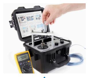
Technician adjusts position of proximity probe to correct for this error
