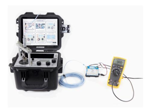
using dynamic calibration. Dynamic calibration often involves a wobble-plate design or in this case, a Model 9100D Portable Shaker Table or 9110D Portable Vibration Calibrator which, essentially, take a 4140 steel target and place it on top of a precision quartz reference accelerometer to simulate actual turbine vibration.
