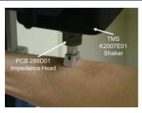
department is using the shaker for Mechanical Response Tissue Analysis (MRTA), a method for measuring bone strength in humans. His research group is focusing on the ulna, the long bone on the little finger side of the forearm. In MRTA data collection, bones are oriented...
