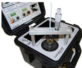
Non-contact displacement sensors, also known as proximity probes, eddy current probes or simply displacement probes, can be checked for accuracy, linearity and frequency response.
