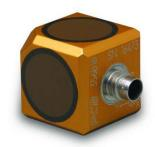
We often get asked the question, "How do I mount a triaxial accelerometer to calibrate the (in plane) X and Y axes, when there is only a single Z axis mounting hole?" Clearly the Z axis stud mount poses no problems, but questions follow such as, "Can I adhesively mount it on the cap
