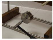
Instrumented impact hammers are a useful and common tool in the structural dynamics and vibration field trouble shooting fields of technology. The hammers, available in sizes from as small as a 0.10 oz (2.9 gm)
